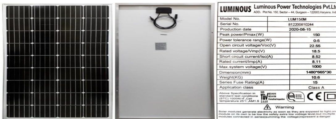
Figure 1. Solar panel used in the experiment is of the monocrystalline type.
