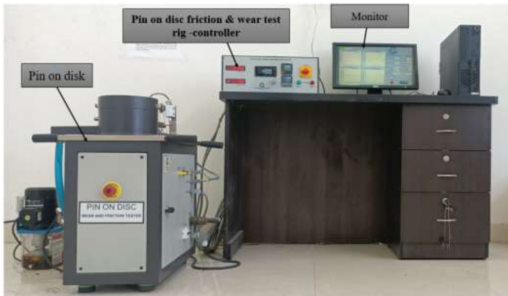
Figure 1: Photograph of the wear testing setup
