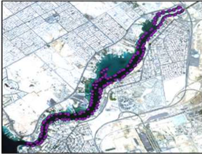
Figure 4. Locations and Distribution of the Calibration MBES Points
