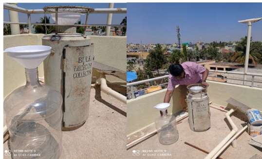
Fig 3: Wet and bulk precipitation collectors and installation at the sites
