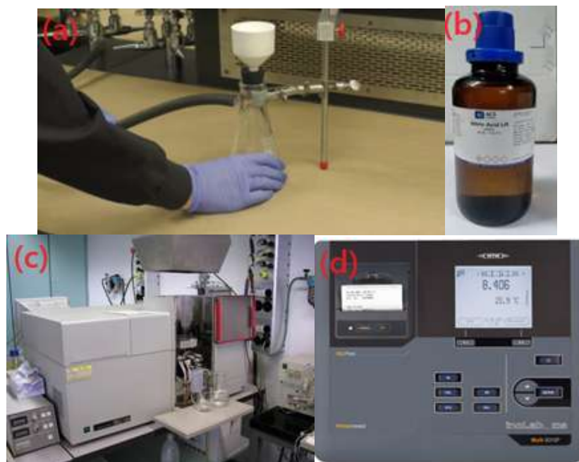
Fig 6: (a) Vacuum filtration system (b) Nitric acid (c) Atomic absorption spectrometer (d) WTW bench top pH meter
