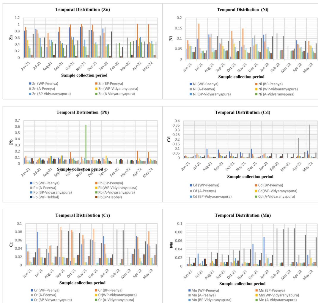
Fig 9: Temporal distribution of Trace metal concentrations measured using rain water samples (Wet precipitation – WP, Bulk precipitation – BP) and Aerosol samples during sampling period
