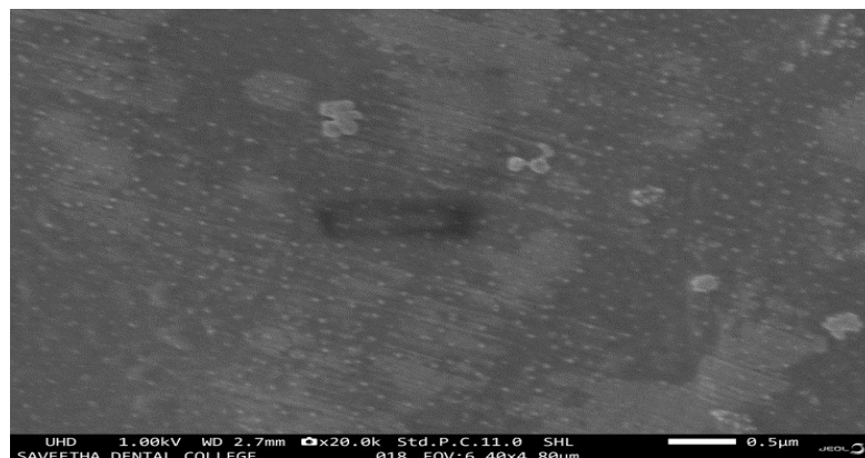
Figure: 3 Scanning Electron Micrograph of Silver nanoparticles synthesized using Phyllanthus acidus fruit
