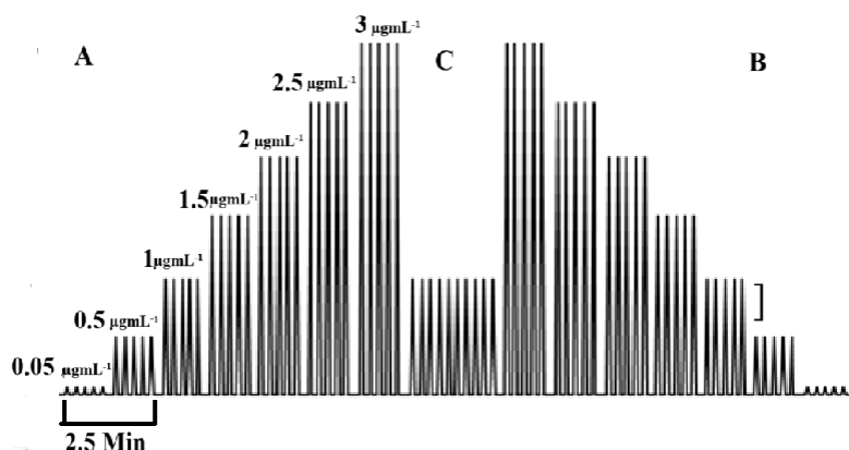
Figure 8. (A). Standard calibration graph for phosphate determination (B). The Peaks obtained by injecting phosphate Standards (C). Ten replicates of 1 µg/mL standard phosphate
