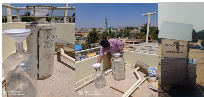
Fig 2: Collectors for wet and bulk precipitation samples and high-volume air sampler
